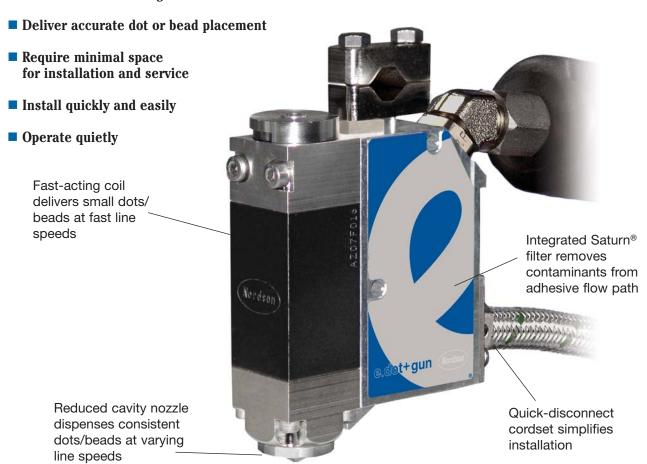
All-electric e.dot+ guns provide precise, high-speed dot or bead placement, quiet operation, a long service life and compact size.
